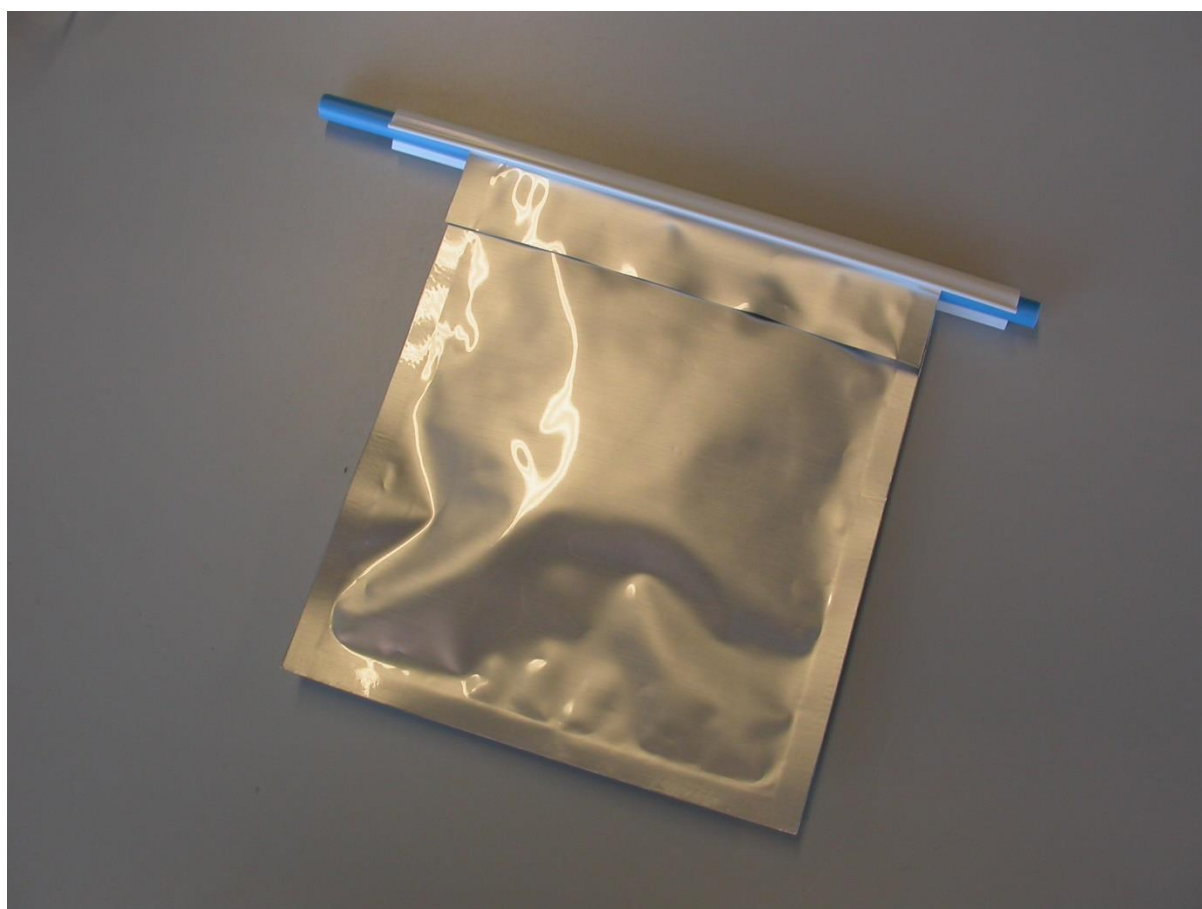
Figure 6: A foil bag sealed for short term storage with a plastic closure strip.
